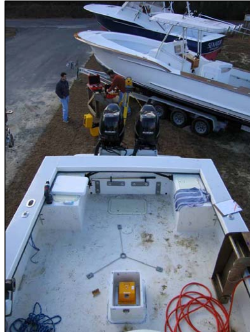
Figure 3. Photo of the centerline and instrument survey by NGS.
